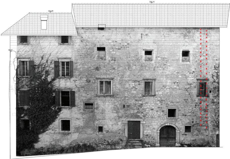
Figure 13. The East front of the Keep: the survey overlaid on the old photograph, with the indication of the height of the stone ashlars in the part to be rebuilt.
