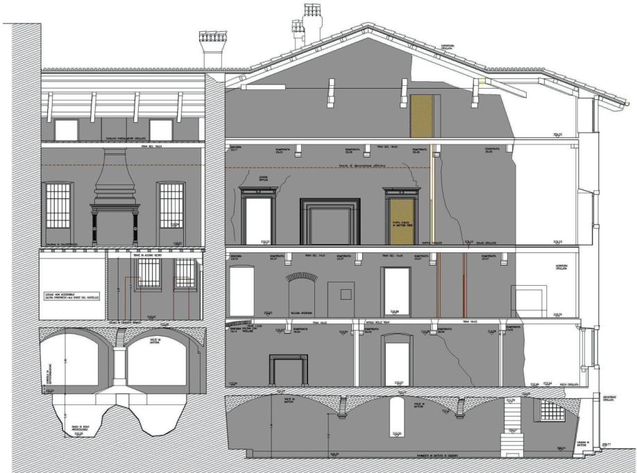
Figure 9. Survey of the Nievo wing: in grey the portion still existent, in white the parts destroyed by the earthquake.
