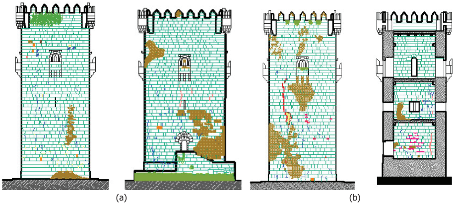
Figure 3. General view of the damages in the tower's facades: (a) southeast and (b) southwest facade and the (c) northwest facade and the (d) interior view of the northwestern wall.
