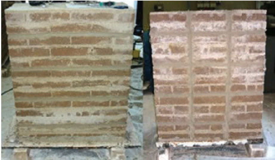
Figure 6. The final aspect of masonry wallets at the end of consolidating process. Sample after "RO" strengthening on the left and after the "RR" one on the right.
