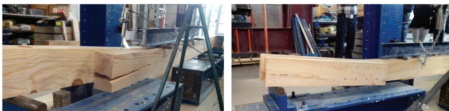
a) Wood splitting in series O
