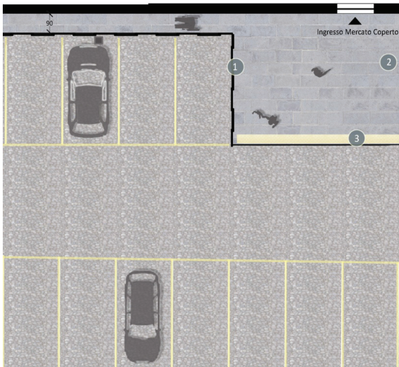
Figure 5. The technical drafting showing the solution to save the path from the cars parking in Piazza Cavagneria; the idea is to maintain no less than 90 centimeters between the wall and the cars in order to allow persons with wheelchair moving without any problem.
