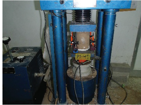
Figure 3. Overview of compressive strength test.
