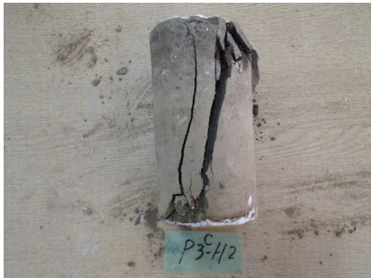
Figure 4. Compressive fracture mode.
