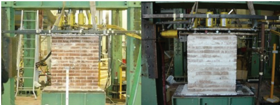
Figure 7. The test device used for vertical compression test (left) and the test device used for shear-compression test (right).
