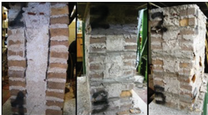
Figure 8. Three-leaf masonry samples after vertical compression tests: on the left the unreinforced ones ("NC"), in the center the ones strengthened through BF arranged only in horizontal bed mortar joints ("RO") and on the right, the ones strengthened through BF arranged both horizontal and vertical bed mortar joints ("RR"). The sample aspect after test shows the effectiveness of the proposed technique.
