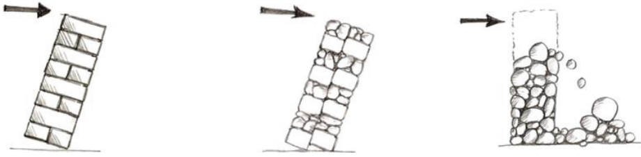
Figure 1. Masonry structural effectiveness directly depends from its quality: good quality masonry subjected to out of plane loads responds like a monolithic body (left), while poor quality masonry is characterized by a chaotic failure (right). For medium quality masonry (center), can be expected a middle behavior.
